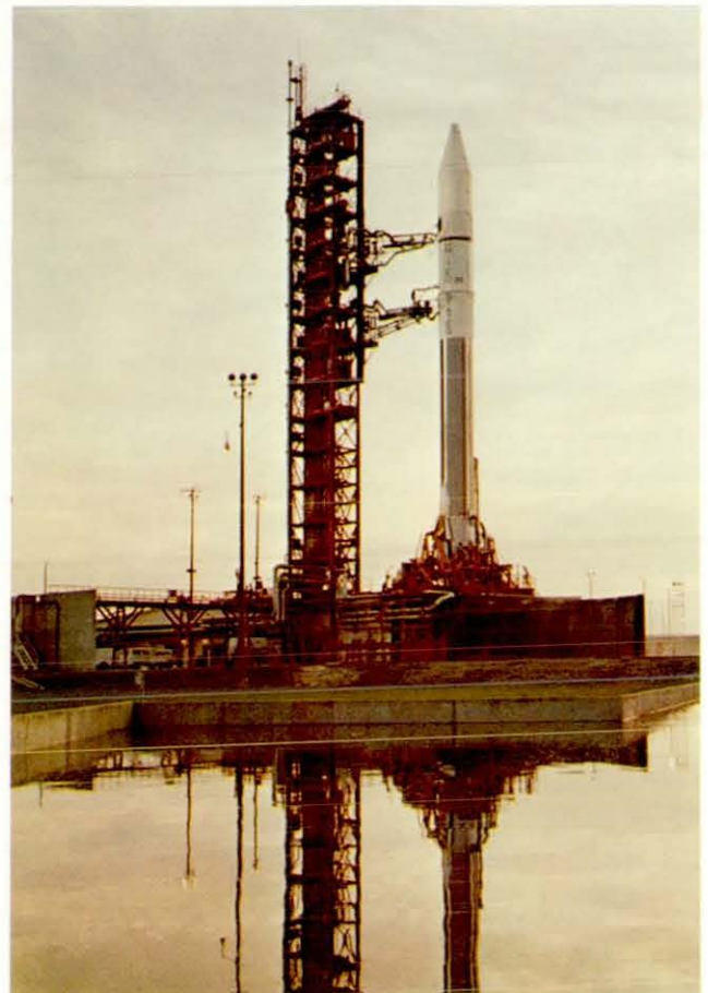
Figure 2-1. The Jupiter mission needed the highest- yet launch velocity of a spacecraft, actually the highest velocity of any man-made object, over 51,500 km (32,000 miles) per hour. This was achieved with an Atlas-Centaur to which was added a third upper stage.
