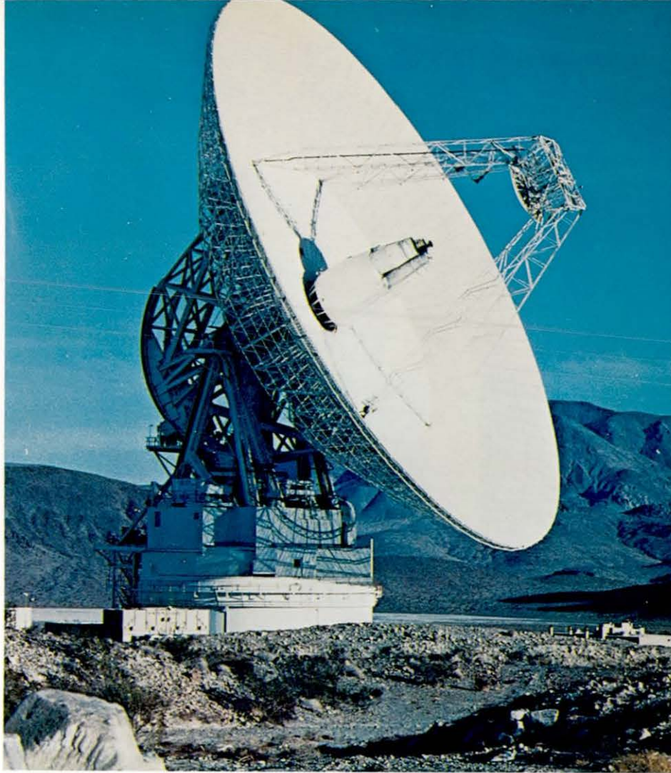
Figure 2-12. Communication with the Pioneer spacecraft at unprecedented distances relies upon the large antennas of the Deep Space Net, such as this one at Goldstone in California's Mojave Desert.
