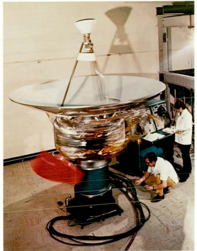
Figure 3-2. The Pioneer spacecraft is stabilized by rotation as shown under test here.
